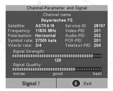
If necessary, you can align your parabolic antenna using the sub-menu «Antenna signal». Turn the antenna to the optimum position in the scales indicating field strength and signal reception quality.
