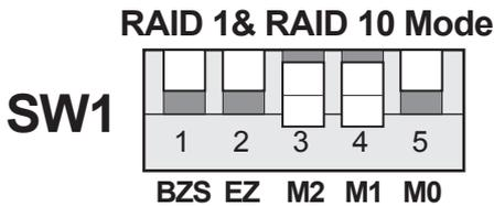
When 2 drives are connected to the HPM-XA, and DIP switch is set to this setting, the 2 drives will be configured as a 2-drive RAID1 array.
