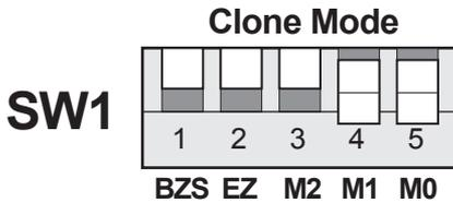
Clone's action is similar to RAID1. However, all of the hard drives will be mirrored. Clone mode is useful especially when users like to copy data from a source hard drive to the drives connected to the HPM-XA.
