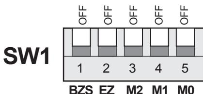
1. Error buzzer function is ENABLED (BZS) when dip switch is in OFF position
