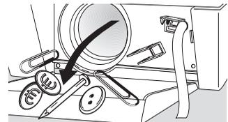
5. Check that you are able to turn the pump wheel at the very rear of the pump housing. (If the wheel rotates with a jerky motion, this is normal.) If you cannot turn the pump wheel, please contact customer service.
