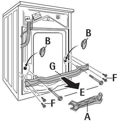
**Attention!** Push in the plug caps so firmly that they engage in the rear panel (this protects the inside of the unit against splash water).
