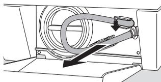
**4.** Place the collecting vessel underneath.
