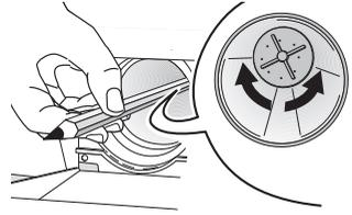
6. Replace the pump cover. Laterally insert the webs on the cover into the guide slots and securely screw on the cover in a clockwise motion.
