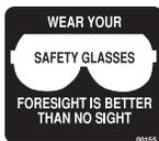
The operation of any snow thrower can result in foreign objects thrown into the eyes, which can result in severe eye damage. Always wear safety glasses or eye shields while operating your snow thrower or performing any adjustments or repairs. We recommend standard safety glasses or a wide vision safety mask worn over spectacles.
