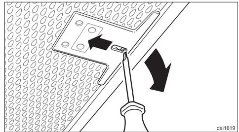
If a grease filter is inadvertently replaced upside down, insert a small screwdriver blade into the slit to disengage the clip.
