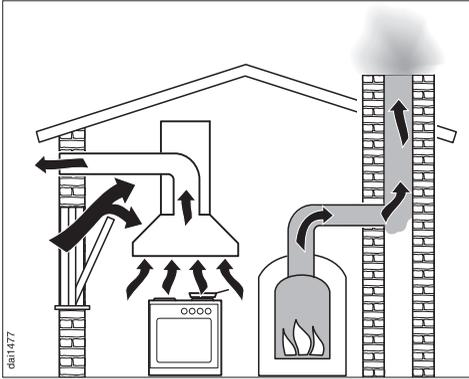
Ventilation can be maintained by air inlets which must not be blocked, in windows, doors and outside wall vents, or by other technical measures, such as ensuring that the cooker hood can only be switched on when the heating appliance is switched off or vice versa. A ventilation brick alone is not generally sufficient to ensure safe ventilation.
