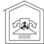
The air is drawn in and cleaned first by the grease filters and then by a **charcoal filter**. The cleaned air is then recirculated back into the kitchen through grilles in the top of the cooker hood extension piece.
