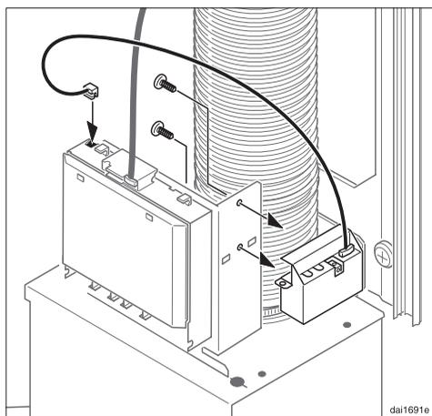
The tower needs to be removed before the control module can be fitted to the fan unit.
