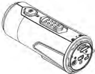
Check that the camera power is turned OFF. Insert a MicroSD card (with the printed side up) into the MicroSD Card Slot with enough finger pressure to keep the edge of the card flush with the card slot opening.
