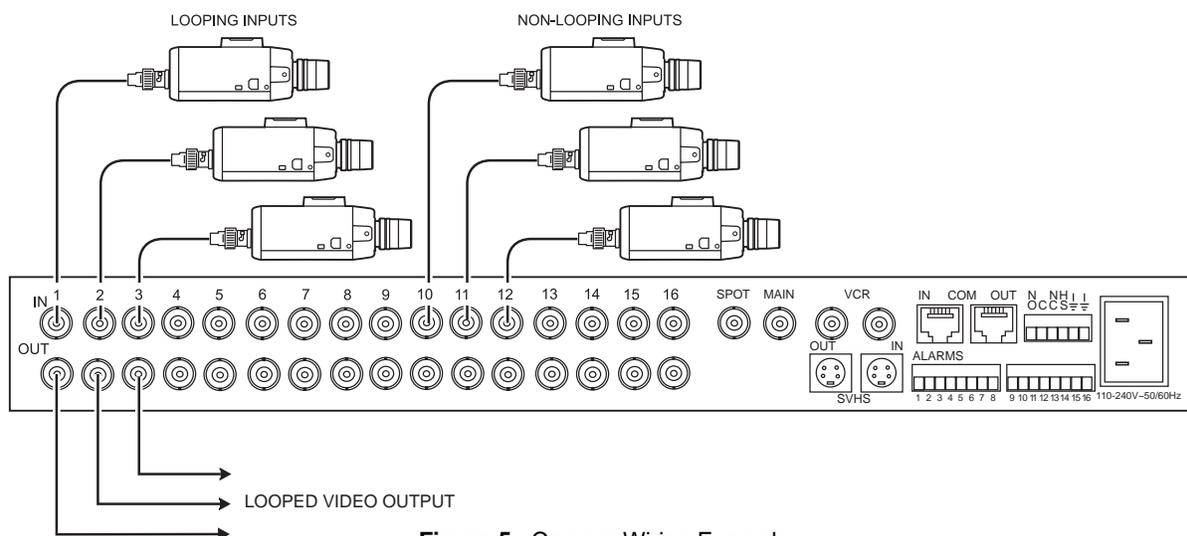
**Figure 5.** Camera Wiring Example
