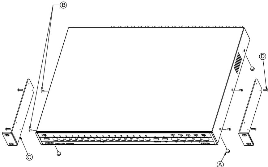
Figure 4. Rack Installation
