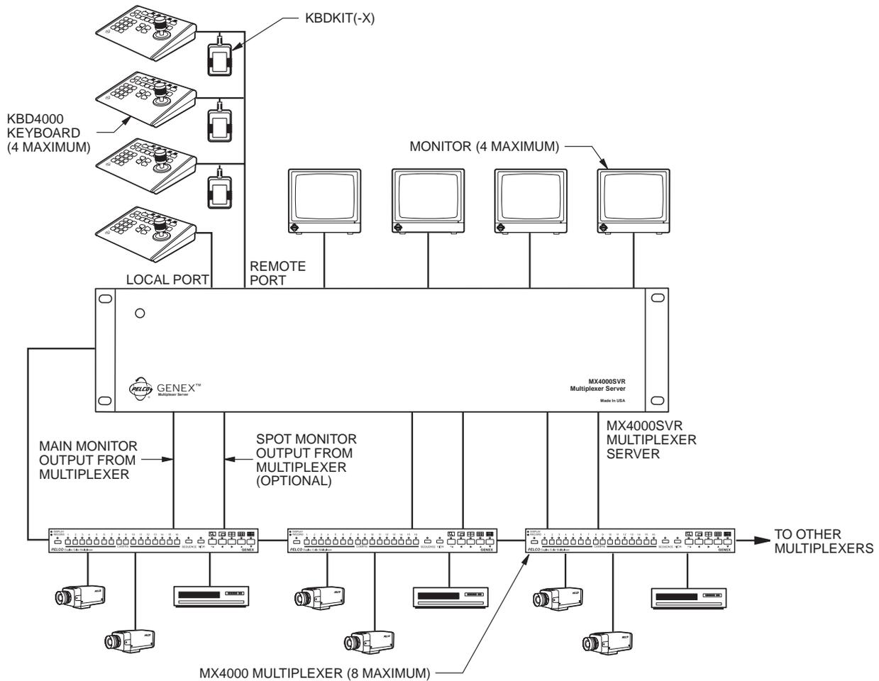
**Figure 3.** Multiplexers with KBD4000 Keyboards and MX4000SVR Server
