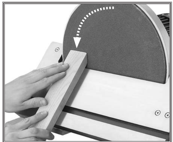
Figure 18. Sanding with table angled.
