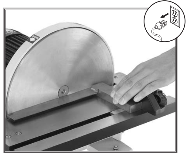
Figure 20. Squaring miter gauge to disc.
