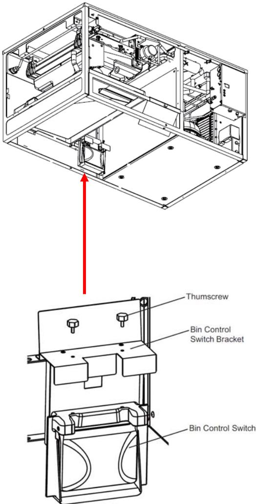
The IM-500SAA uses a mechanical bin control located on the right rear side of the ice drop zone. This control will open when ice pushes against the switch, if the switch stays open for more than 10 seconds the machine will start the bin control cycle, starts and the machine will shut down after the next defrost cycle.
