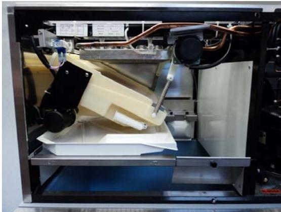
The moveable water pan assembly includes the water plate, reservoir pan, and pump motor assembly. Tension springs connect two cam arms to the water plate assembly. An actuator motor rotates the cam arms to raise and lower the water pan during the ice making cycle.
