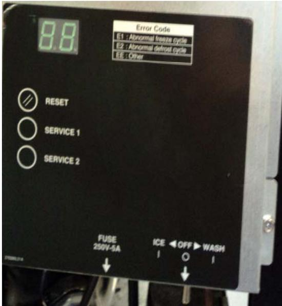
The control switch is marked “ICE-OFF-WASH” and is located on the upper right front of the unit.
