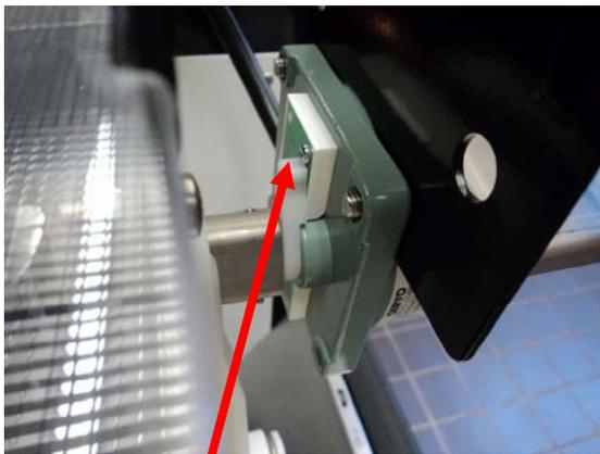
**Hall IC Switch is located on the motor backside. (Magnetic Switch)**
