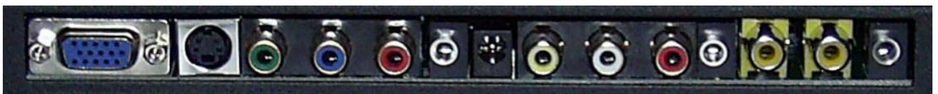
VGA S-Video Y Pb Pr PC 12V Video 1 L R Line Video Vdeo2 IR sound DC IN OUTPUT Ext.
