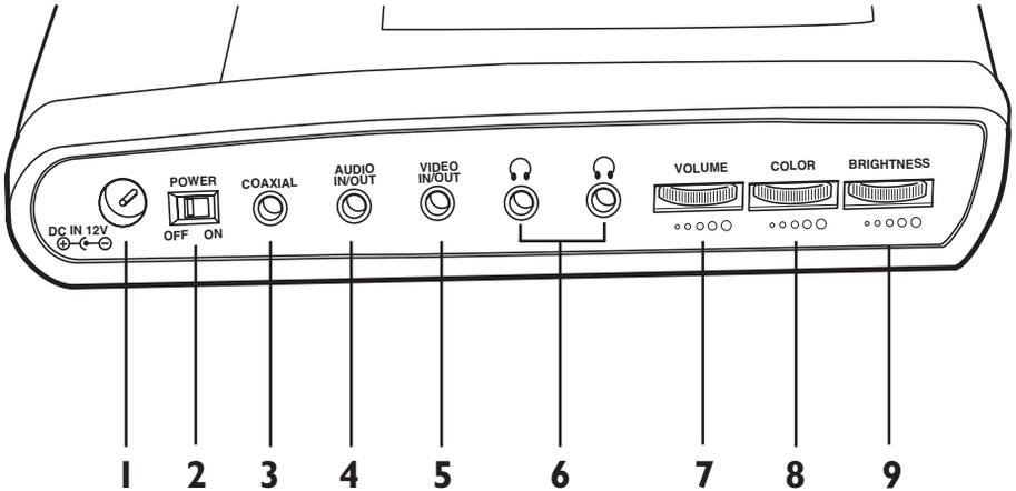
1. **DC IN power jack** — Connect the power supply here.
