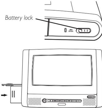
1. Slide the battery lock on the left side of the unit to the OPEN position to open the battery compartment.
