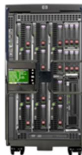
Figure 1-7 is an illustration showing the location of the device bays, optional DVD drive, Insight display, and Onboard Administrator at the front of the HP BladeSystem c3000 Enclosure.
