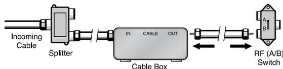
4 Connect another cable between the other OUT terminal on the splitter and the A-IN terminal on the RF (A/B) switch.
