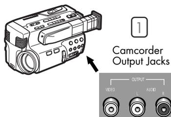
2 Connect a set of audio cables between the AUDIO IN jacks on the TV and the AUDIO OUT jacks on the camcorder. If you have a mono Camcorder, connect L(mono) to the Camcorder audio out using only one audio cable.
