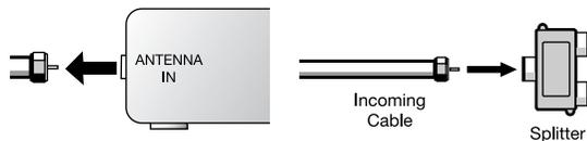
2 Connect a coaxial cable between an OUT terminal of the splitter and the IN terminal of the Cable box.
