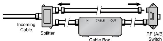
5 Connect the last coaxial cable between the OUT terminal of the RF (A/B) switch and the ANT 1 IN (CABLE) on the TV.
