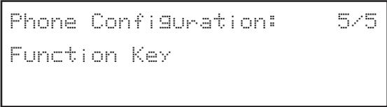
2. The telephone prompts the user to press the desired Function Key. When the Function Key is pressed, the current assignment for the key is displayed in the LCD.
