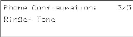
2. The current ring tone is displayed. Use the ↑ and ↓ keys to access the desired ring tone. As you scroll through the selections, the ring tone can be heard for three seconds. When the desired ring tone is displayed, press **SELECT** key.
