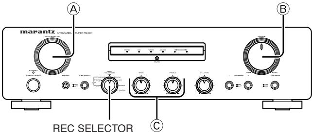
Control used for operating the tape deck.
