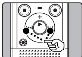
While the recorder is during stop mode, press and hold the ▶▶ or ◀◀ button.
