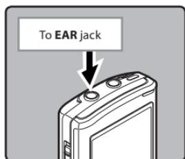
An earphone can be connected to the EAR jack of the recorder for listening.
