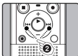
2 Press the ►►► or ◀◀◀ button to select the index or temp mark to erase.
