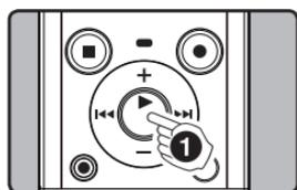
**1** While the recorder is during stop mode, playback mode or recording mode, press the ► OK/MENU button for 1 second or longer.
