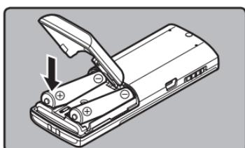
② Insert size-AAA alkaline battery, observing the correct  $\oplus$  and  $\ominus$  polarities.
