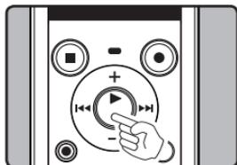
While the recorder is during recording mode, press the **▶ OK/MENU** button.
