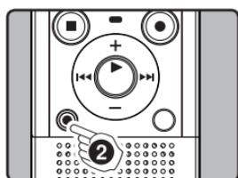
**2** While the recorder is during stop mode, press the ERASE button.
