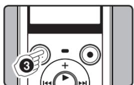
**3 Press the STOP (■) button to stop recording.**
