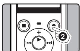
**2 Press the REC (●) button to start recording.**
