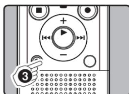
3 While the index or temp number appears for approximately 2 seconds on the display, press the ERASE button.
