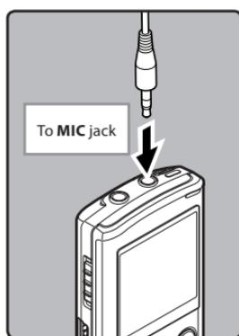
The external microphone and other devices can be connected and the sound can be recorded. Connect as follows by the device to be used.
