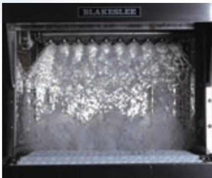
Top and bottom mounted water jets provide torrential cleaning & rinse action.
