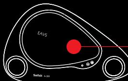
On top of the Portable speaker system press down the EAVS woofer enclosure to release it and to turn on the speaker system. The speaker system will not work until the woofer enclosure is open.
