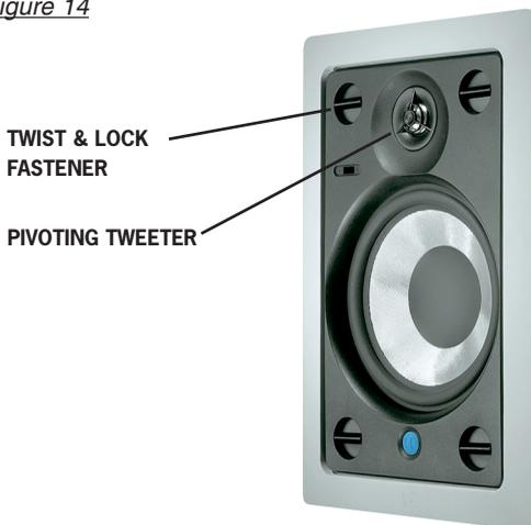
3. Insert the speaker grille by placing it over the speaker baffle and aligning its edges in the frame. Press gently into place, taking care not to scratch the frame finish. The grille is made from pliable, non-rusting aluminum. If the grille seems loose in the frame, gently remove it, carefully bend a slight flare on the outer edges, and re-insert into the frame.
