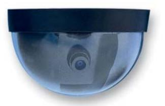
Our 1/3" B/W CCD dome camera with smoked housing can be mounted on the ceiling and offers unobtrusive surveillance. It can be rotated 360 degrees for maximum viewing angle and tilted +/-90°. It features .02 lux sensitivity with 420 lines of resolution and a 3.6mm wide angle lens with built-in electronic shutter. A 12V DC power supply is included.
