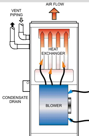
NOTE - The vent piping and condensate drain can be moved to the other side of the unit. Vent piping and drain must be installed on the same side of the unit with each other unless optional Condensate Trap Alternate Location Kit is used.
