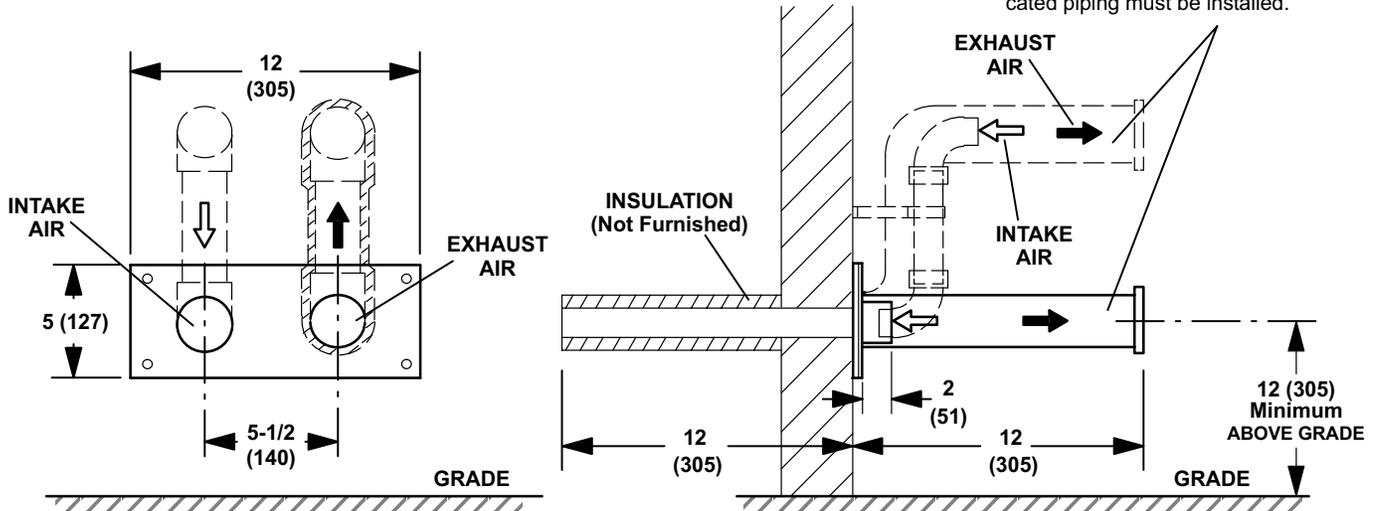
**WTK WALL ASSEMBLY TERMINATION KIT WITH FIELD FABRICATED ABOVE GRADE EXTENDED CLEARANCE**
