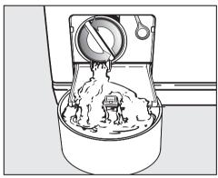
■ Place a suitable container under the access flap.
