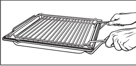
The handles are used to take the baking trays or the roasting pan in and out of the oven.
