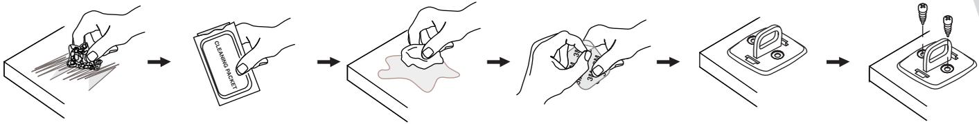
**NOTE:** When using the adhesive backing, apply at room temperature - 60°F (16°C), and allow it to bond for more than 24 hours. Not recommend for to use in outdoor or high humidity environment. Bonding to glass, ceramic tile, water-absorbent materials, copper, brass, or plasticized vinyl without primer surface are not recommended.
