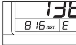
An “E” (for English) or an “M” (for metric) will appear in the lower right display. Press the Speed increase button to change the unit of measurement, if desired.
