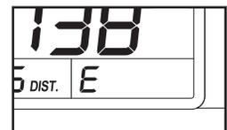
key. Next, hold down the Stop button, insert the key into the console, wait until you hear a tone, and then release the Stop button. An "M" for metric kilometers or an "E" for English miles will appear in the lower right display. Press the Speed increase button to change the unit of measurement if desired. When the desired unit of measurement is selected, remove the key and then reinsert it.
