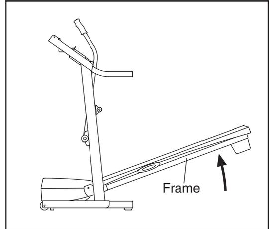
2. Move your right hand to the position shown and hold the treadmill firmly. Using your left hand, pull the latch knob to the left and hold it. Raise the frame until the hole in the frame is aligned with the latch pin. Slowly release the latch knob; make sure that the latch pin is fully inserted into the hole in the frame.
