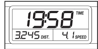
**The lower right display**—The lower right display can show the approximate number of calories that you have burned and the speed of the walking belt. The display also shows your heart rate when you use the pulse sensor (see step 6).
