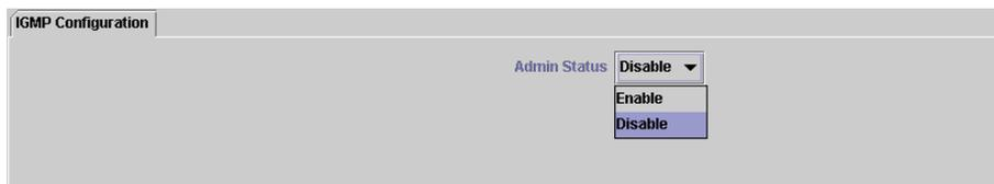
**NOTE:** As IGMP Snooping only operates under 802.1Q VLAN mode, please change VLAN mode from Port Group VLAN to 802.1Q VLAN before enabling IGMP Snooping.
