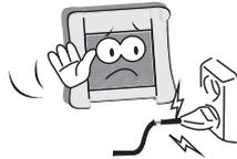
Do not connect excessive sockets in parallel or share the same socket by multiple plugs to avoid fire hazards.
