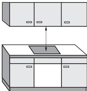
When two or more appliances are installed together below a cooker hood, e.g. a gas wok and a ceramic hob, which have different safety distances given in the installation instructions, you should select the greater distance of the two.
