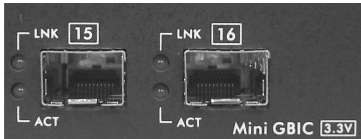
Figure 2-4. Combo SFP Slots port LED Indicators
