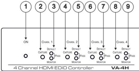
Figure 1: VA-4H 4-Channel HDMI EDID Controller Front Panel
