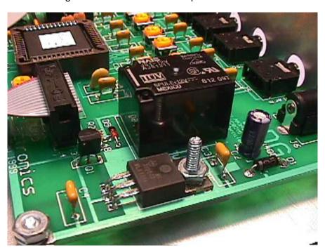
Install the 2N3904 transistor, Q1. Note the correct orientation.
