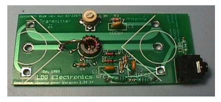
Install the ceramic capacitor, C3 100pf 1KV.
