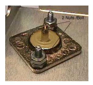
Place the PC board onto the SO-239s. Align the 1/8" jack with the hole in the enclosure. Once this is in place, you may tighten the nuts that are underneath the PC board. You do this by pressing the board down on the nuts while turning the screw. Repeat with the other three screws.
