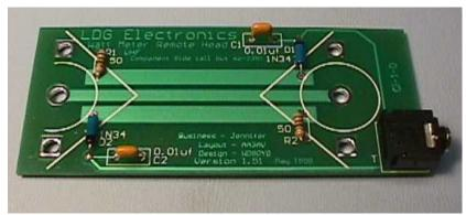
Install the diodes, D1 and D2. Note the band polarity.
