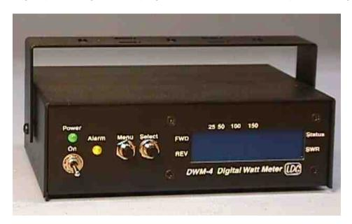
**Introduction:** The DWM-4 is a four channel, microprocessor controlled RF wattmeter. It consists of two main parts, the display unit and the remote sensor. The display unit has a 2 by 16 backlit LCD module that provides the user with information about the RF that is being sampled by the remote sensor. The user can simultaneously view forward power, reverse power and swr on the same display for instant analysis of the antenna system.
