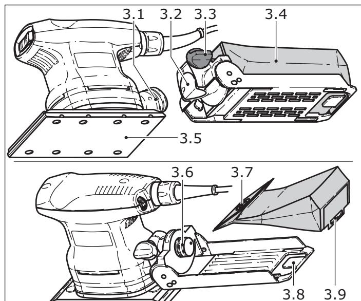
The machines are fitted with inbuilt extraction as standard. The sanding dust is extracted through
