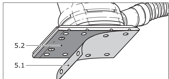
Simply press the abrasive (5.1) onto the sanding pad (5.2) and pull it off again after use.
