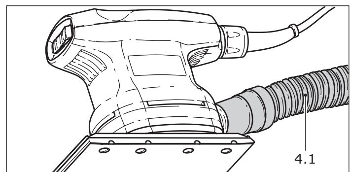
In order to avoid frequent changing of the turbo-filter when carrying longer sanding jobs, it is possible to connect a Festool extractor to the unit instead of using inbuilt extraction.
