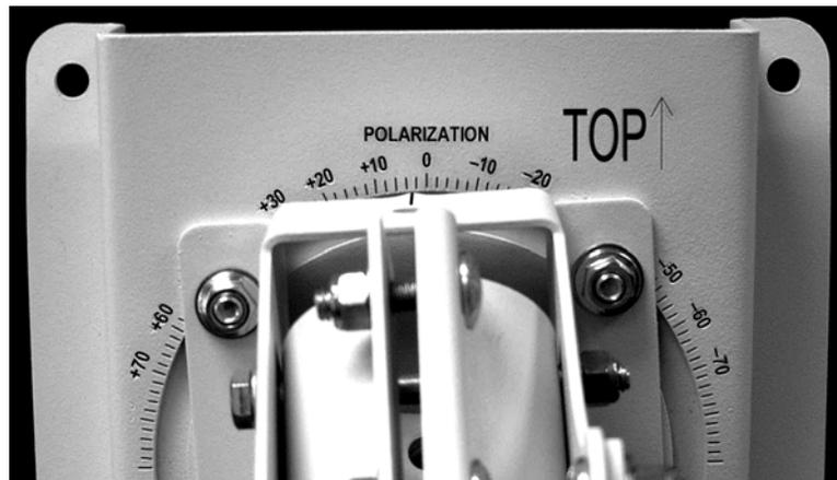
Figure 12: Locating the polarization scale
