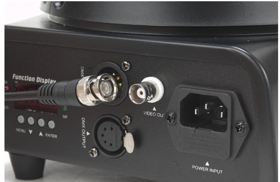
Use a BNC video cable or RCA video cable, with RCA/BNC adaptor, to connect to a video converter or source such as Elation's EPV Image VSC.
