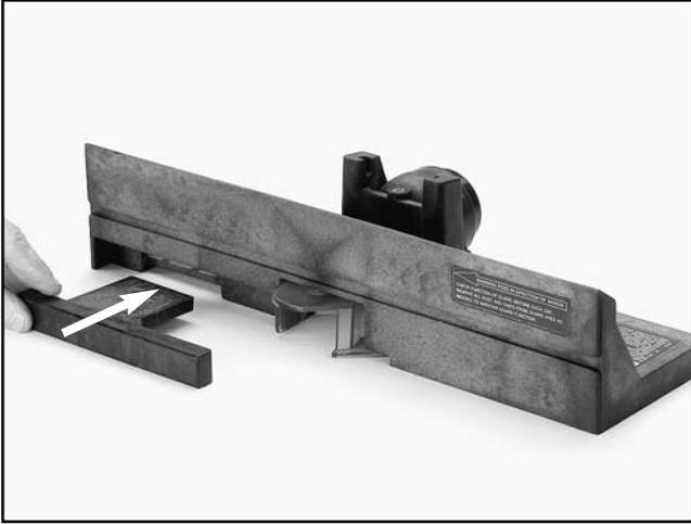
**Figure 13.** Installing the pocket jointing fence.
