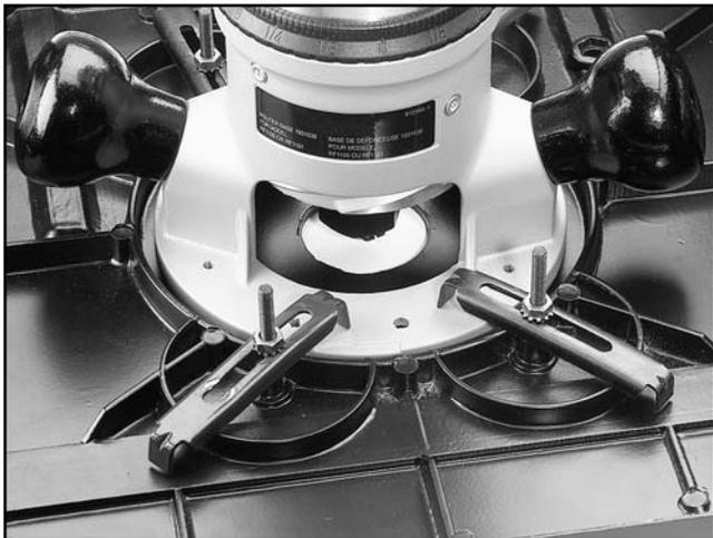
**Figure 10.** Correctly clamped router.
