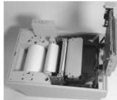
paper feed roller inside the print mechanism then the paper will automatically advance to proper position (paper exit of print mechanism). In case there was a slip at the insertion of the leading end of paper roll and you want to keep same heading clearance, you may press the FEED button to advance the paper to position.
