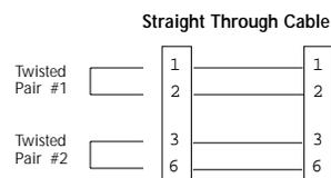
The two active pairs in a 100BASE-TX network are pins 1 & 2 and pins 3 & 6. Use only dedicated wire pairs (such as blue/white & white/blue, orange/white & white/orange) for the active pins.
