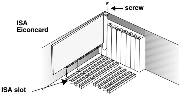
Figure 2. Inserting the Eiconcard C2x.
