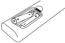
Remove the battery cover on the rear of the Remote Control, and insert two (size AAA) batteries with **+** and **-** matched correctly.
