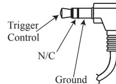
*Note: The Data, Power Control and Trigger Connecting Cable is available from the McIntosh Parts Department:*
