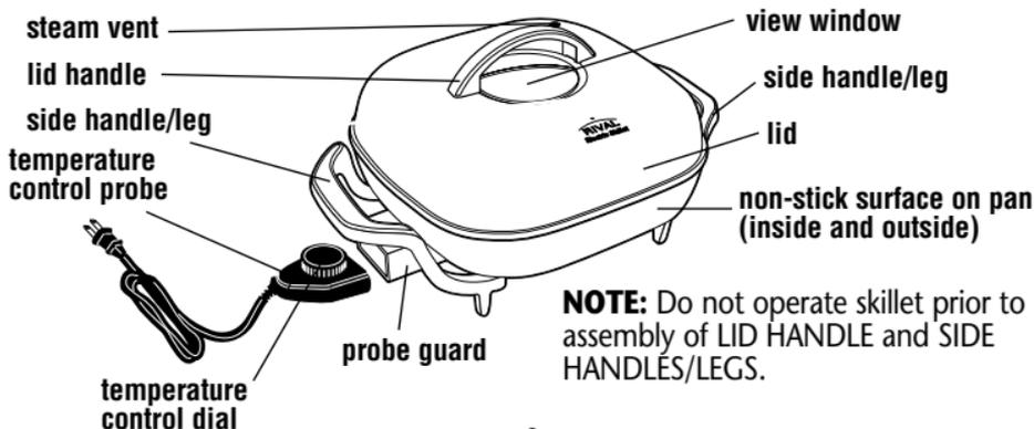
**NOTE:** Do not operate skillet prior to assembly of LID HANDLE and SIDE HANDLES/LEGS.
