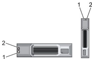
Figure 8. SCv2000/SCv2020 Drive Indicators
