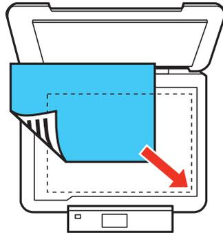
**Note:** You can place multiple originals on the scanner glass. Just make sure they are at least 0.20 inch (5 mm) away from each other and from the edge of the scanner glass.
