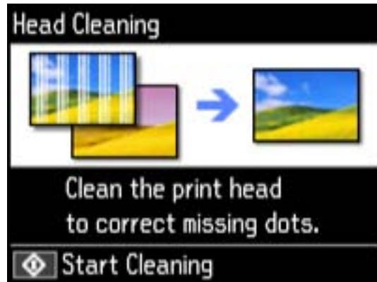
7. Press the
