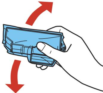
**Caution:** Do not shake the cartridges after opening the packages, or ink may leak.
