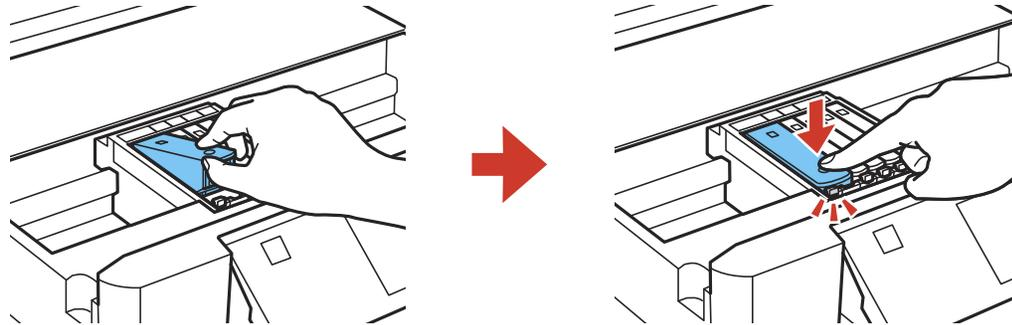
10. Once you replace all the cartridges that need replacing, close the scanner unit.
