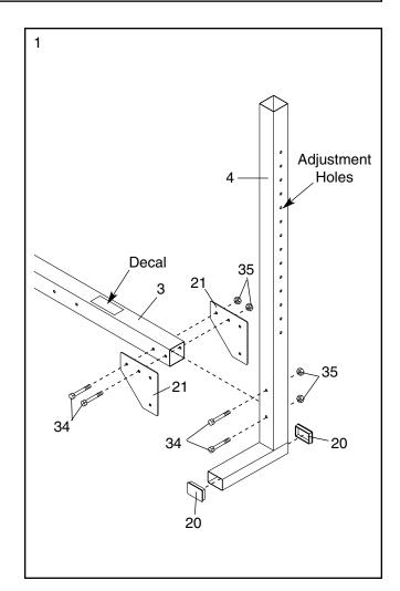
Attach the Frame (1) to the Crossbar (3) with two M10 x 95mm Bolts (34) and two M10 Nylon Locknuts (35). Do not tighten the Nylon Locknuts yet.
