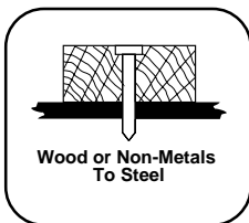
Fasten wood or nonmetals to concrete or steel.
