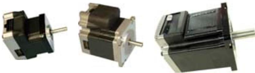
The DSM family use a NEMA17, NEMA23 or NEMA34 1.8° high torque motor combined with a microstepping drive, and accept up to 14 resolution settings from 1/2 to 256 microsteps per step. Setup parameters can be changed 'on-the-fly' or downloaded and stored in non-volatile memory with the use of a simple user interface program which is provided, eliminating the need for external switches or resistors. The versatile, compact DSM is available in multiple configurations to fit various system needs.
