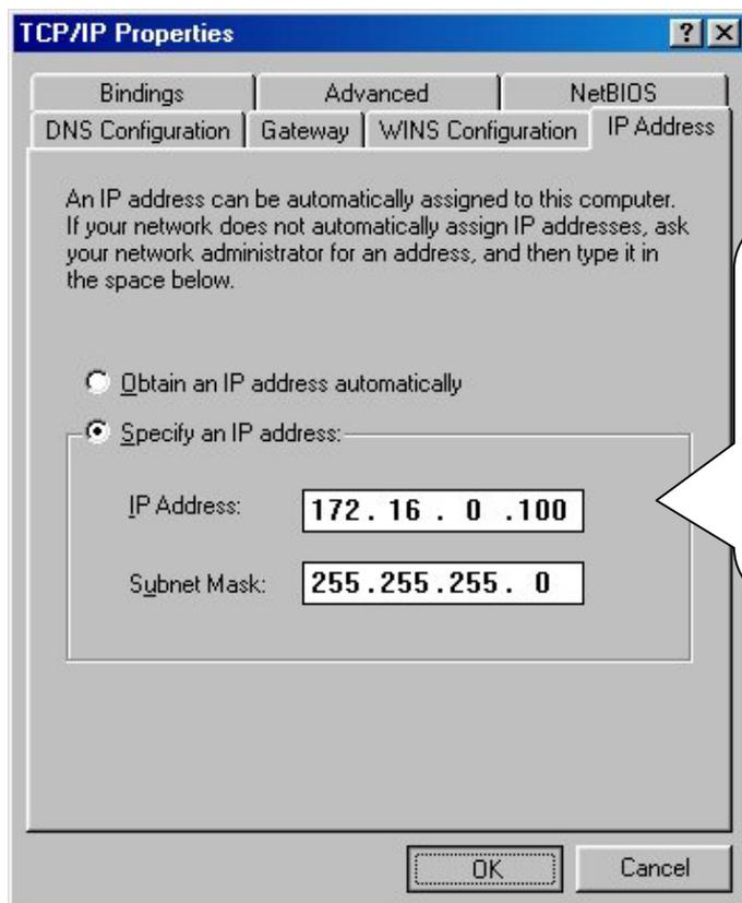
Set "IP Address" and "Subnet Mask" on [IP Address] Menu. In this case, IP Address entered on "IP Address" must have same Network Address of IP Address of AP assigned for NAT.(Refer step ①.)
