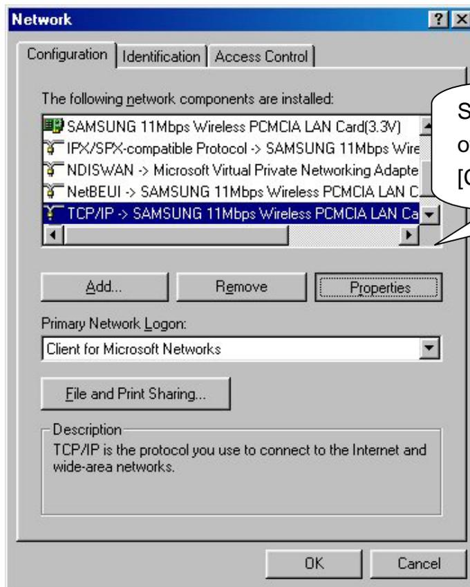
Select "TCP/IP" [Properties] of LAN Adapter to use on [Configuration] Menu.
