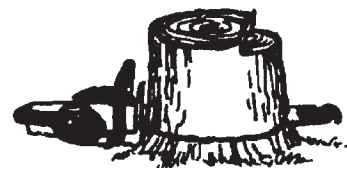
KICK GUARD® PROTECTS CHAIN FROM GROUND WHEN FLUSH CUTTING.
