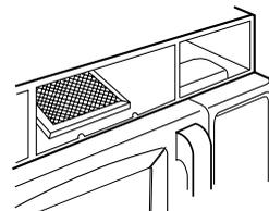
6. Slide the bottom of the vent cover into place. Push the top until it snaps into place. Replace the mounting screws. Turn the power back on at the main power supply and set the clock.
