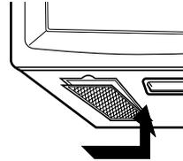
NOTE: **Do not** operate the hood without the filters in place.
