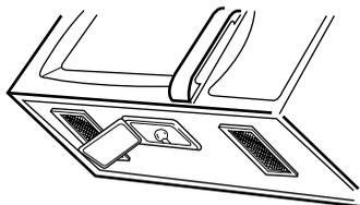
3. Replace bulb with 30 watt appliance bulb.
