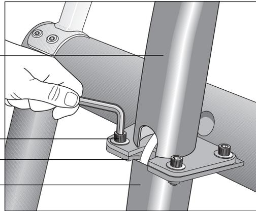
7. **Secure the console assembly to the base frame support.** Diagram 4. Place a washer (B) on each of 4 screws (A). Align the mounting holes and insert the screws through the upper and lower bracket. Use the hex key provided to alternately tighten each screws until all four screws are secure.
