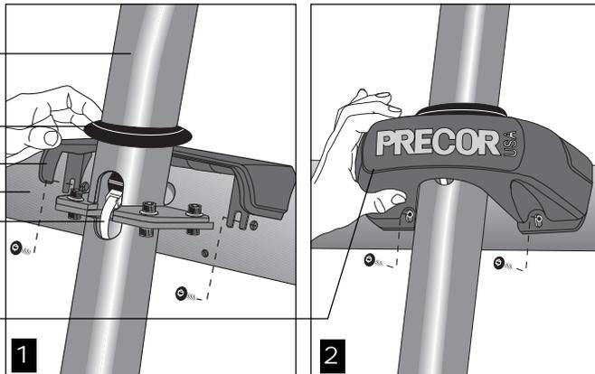
8. **Install the bracket covers.** Diagram 5. Remove the 2 bracket covers, the split rubber grommet and 4 screws (C) from the Hardware kit. Then, take the following steps:
