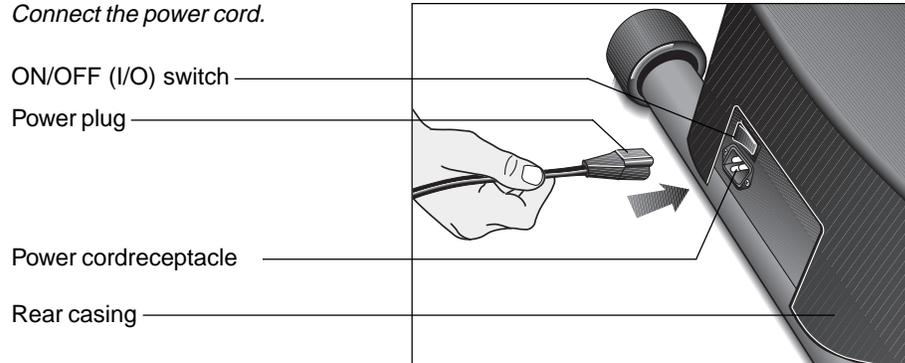
11. **Connect the power cord.** Diagram 7. Insert the power plug's connector into the receptacle at the rear of the base assembly.
