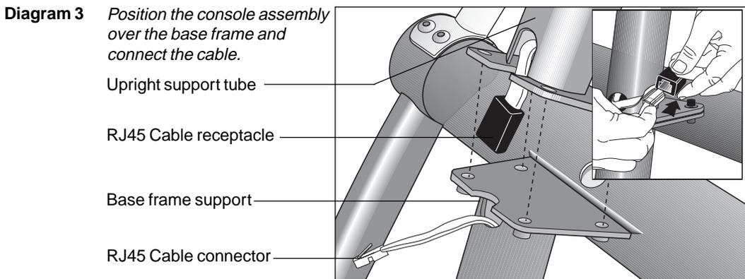
5. **Position the console assembly over the base support.** Diagram 3. Remove any tape that secures the RJ45 cable. Have an assistant hold the upper support tube over the base frame support (display console must face the foot pedals) while you connect the cable and align the bolt holes.
