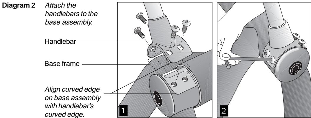
4. **Attach a handlebar to one side.** Diagram 2. Take the following steps:
